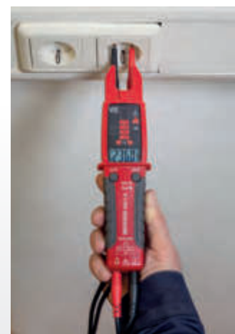
One-hand operation for voltage measurement
