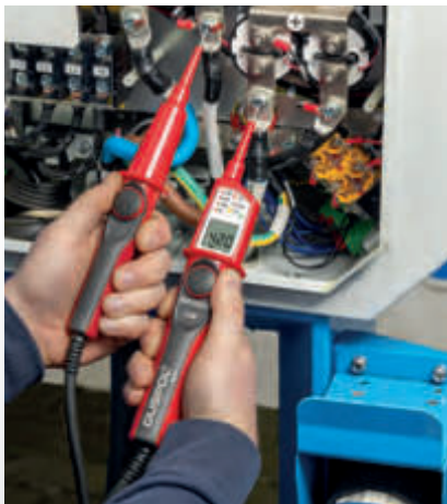
Testing the output voltage of a DC charging device
